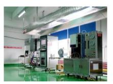
Water Heater Integrated Automatic Testing Equipment
